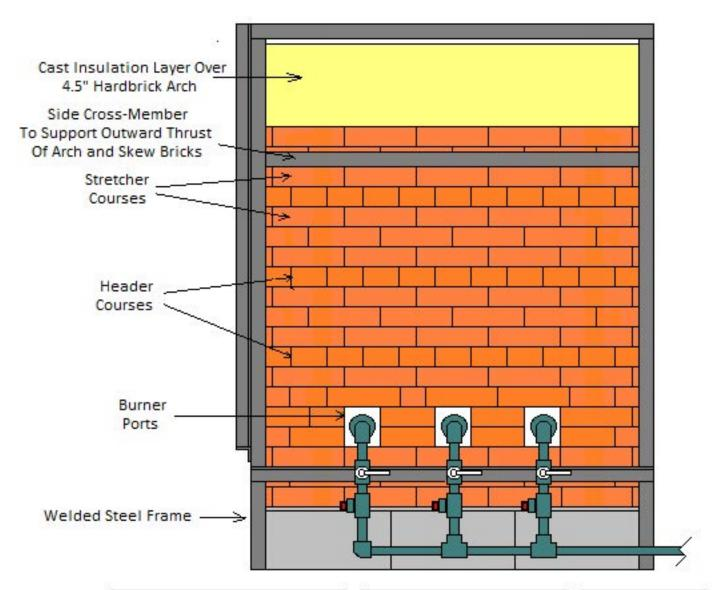
Downdraft Crossdraft Soda Kiln Propane-Fired, 30 Cu. Ft. 20 Cu. Ft. Stacking Space Vince Pitelka, 2019 Scale Approx. 12:1 SIDE VIEW
