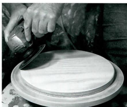
g. Sand a beveled outer edge on the bats with a sanding disk on an angle grinder.
