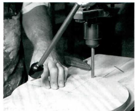
e. Drill appropriate bat-pin holes.
