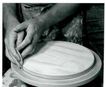
h. Sand the vertical surface of the bats.
