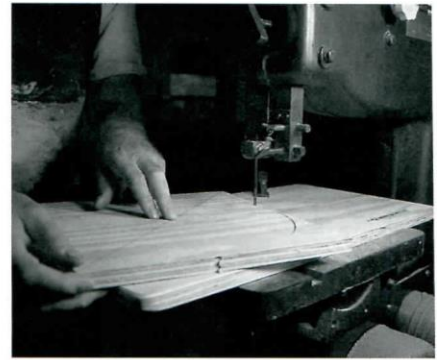
b. With gentle downwards pressure on the center point, rotate the square to cut a perfect circle.
