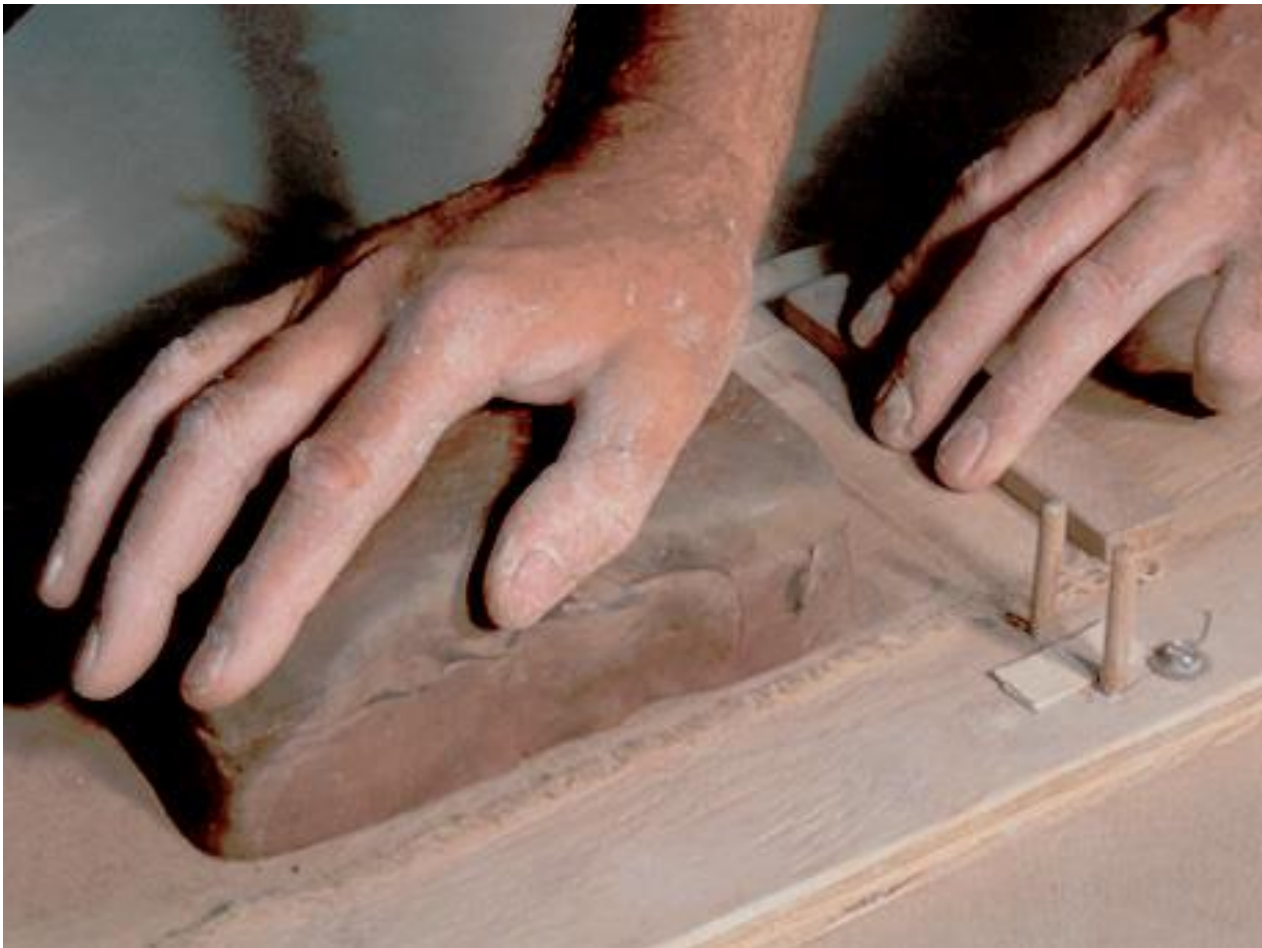
Veneer-slicer in use. Patterned loaf on canvas strip being pulled through cutting wire. Note wood "handle" on canvas strip.
