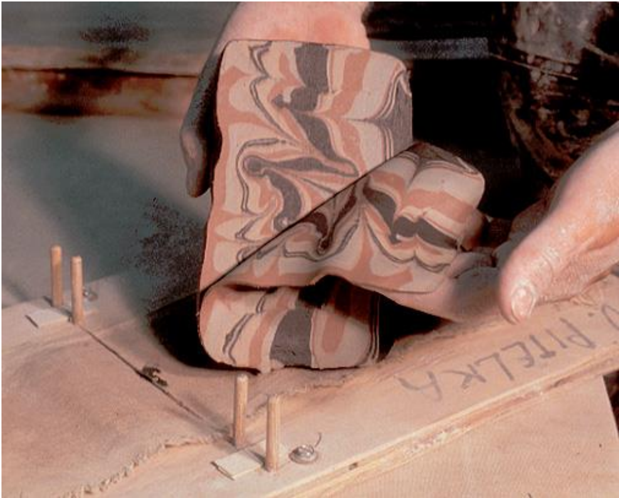
Very thin lamination being peeled from loaf after cutting. Note residue on cutting wire. Always remove that residue after each cut.
