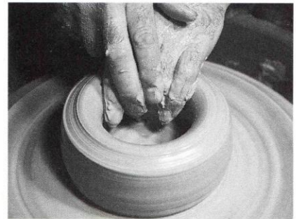
c. Widen the bottom using the "claw" motion, and compress the bottom.
